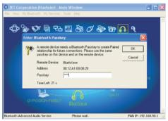
iv. After input correct PIN key, the Bluetooth connection will be built, and you can use the BlueWave speaker now. You can see also a check symbol displayed by the BlueWave icon and a dotted line connecting with the central sphere.
