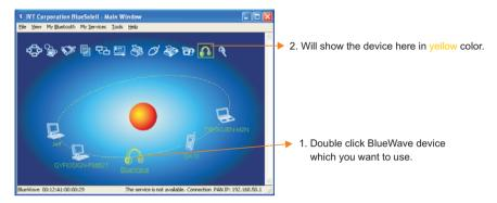
viii. DoubleClick the device's function on the upper right conner which you want to use. Then IVT will show out a window to ask you fill up the PIN key. Please Key in the correct PIN key 0000.
